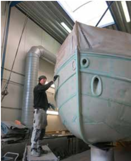
Applying the two component filler
