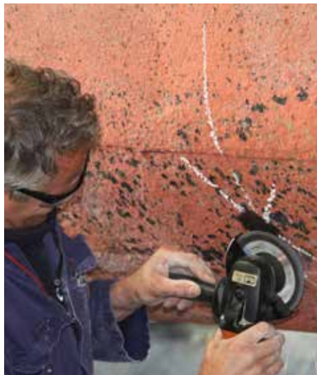
Preparation before measuring the thickness of the hull
